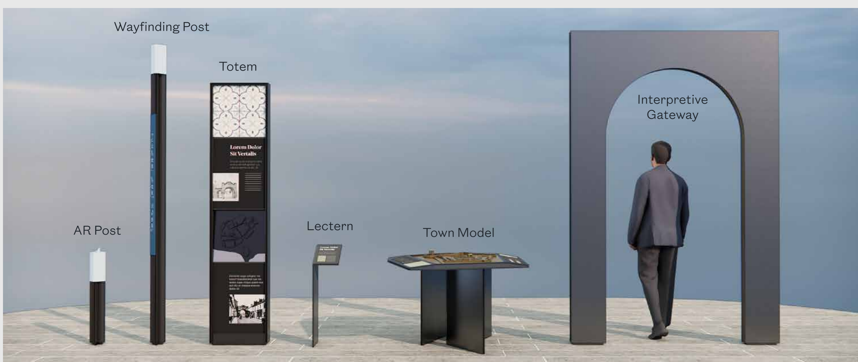
Above Suite of proposed interpretation furniture that will be located around the town walls.
